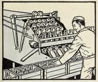
In a bottling plant, nearly all of the work is done by machinery. This is one of the bottlewashing machines.
